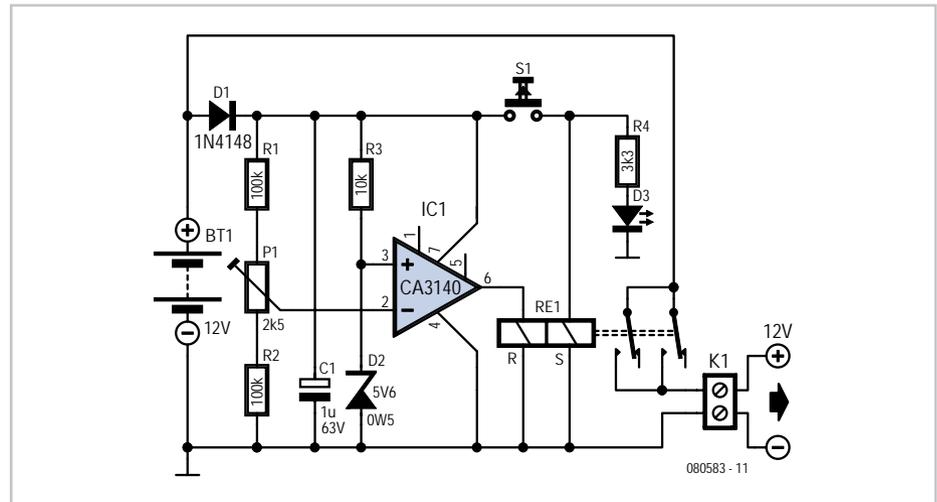
the battery voltage rises above the reference voltage again, the reset coil will no longer be powered and the current consumption drops back to about 2.5 mA.
